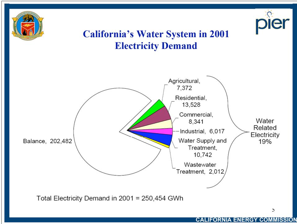
**This chart show how and where power is used in the State's water systems. The CEC's water and energy research is designed to obtain a greater understanding of how this energy is used within these sectors, and how it can be used more efficiently.**
